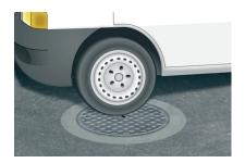
Ceiling of manholes should be quickly efficient, to resist to the weight of cars passing over it. traditional site-mixed sand/cement bedding mortar will crack and crumble under traffic loads, resulting in premature failure of the cover and frame.
